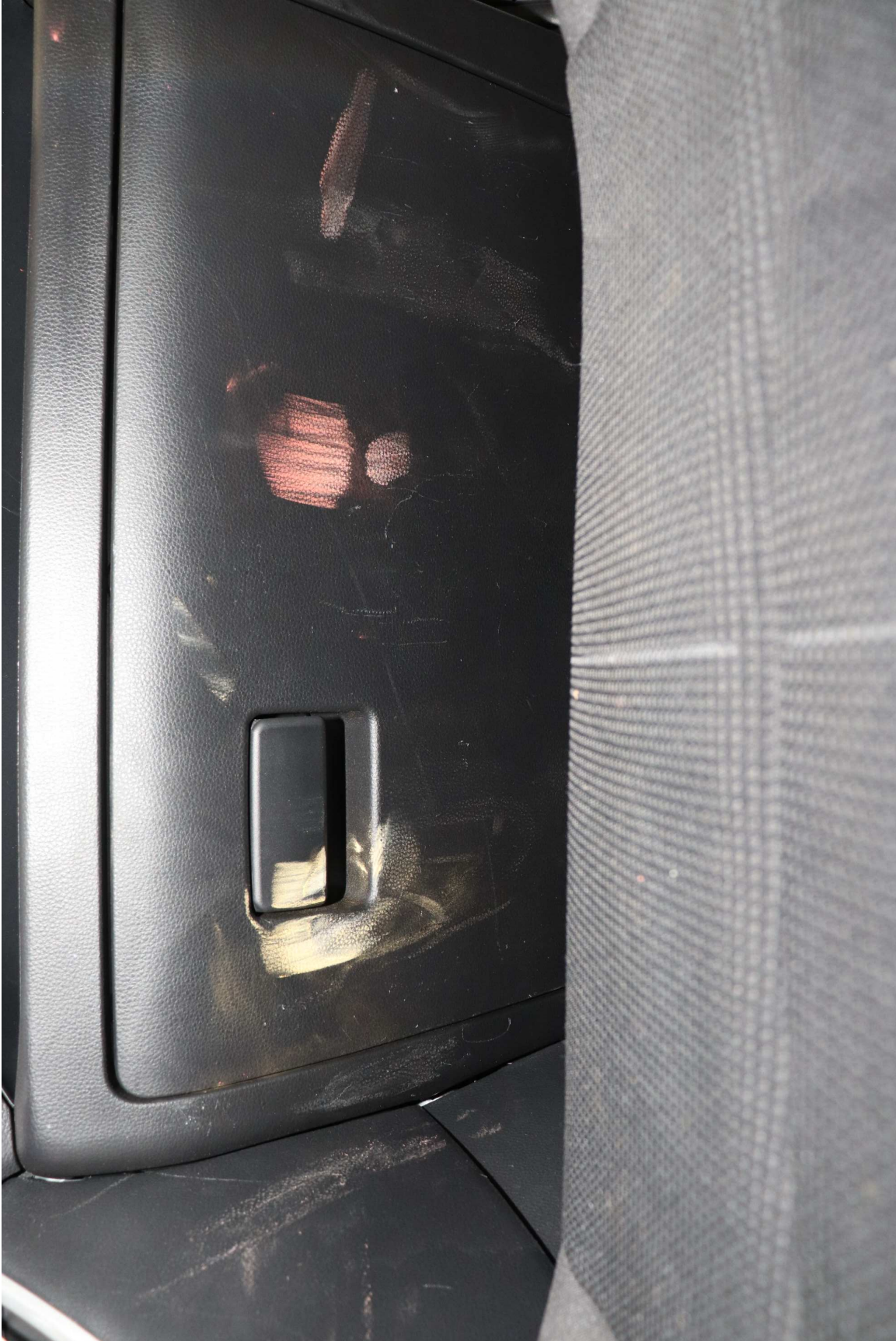
Photo No. 61. Post-Test Passenger Dummy Knee Contact
