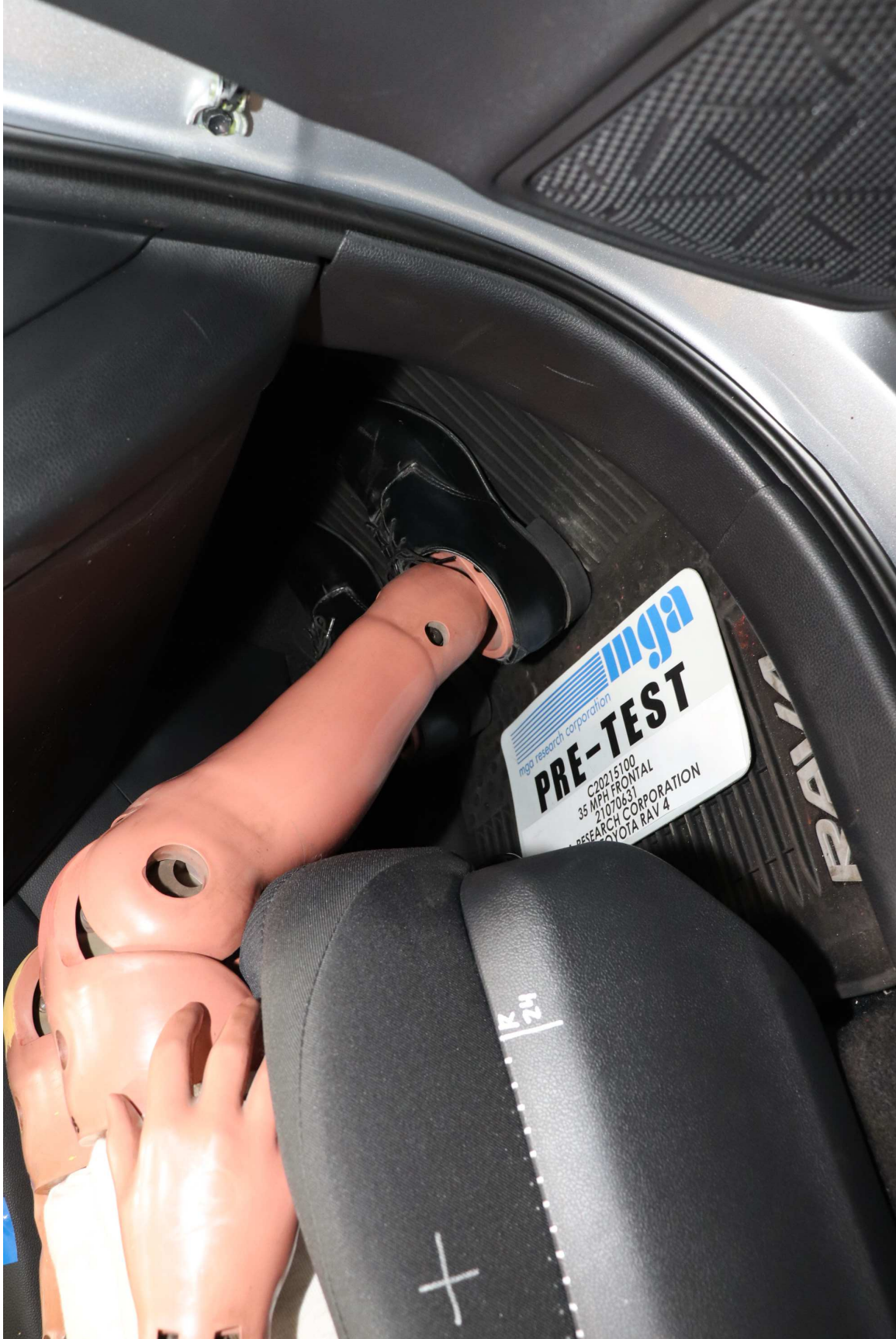
Photo No. 56. Pre-Test Passenger Dummy Feet Position
