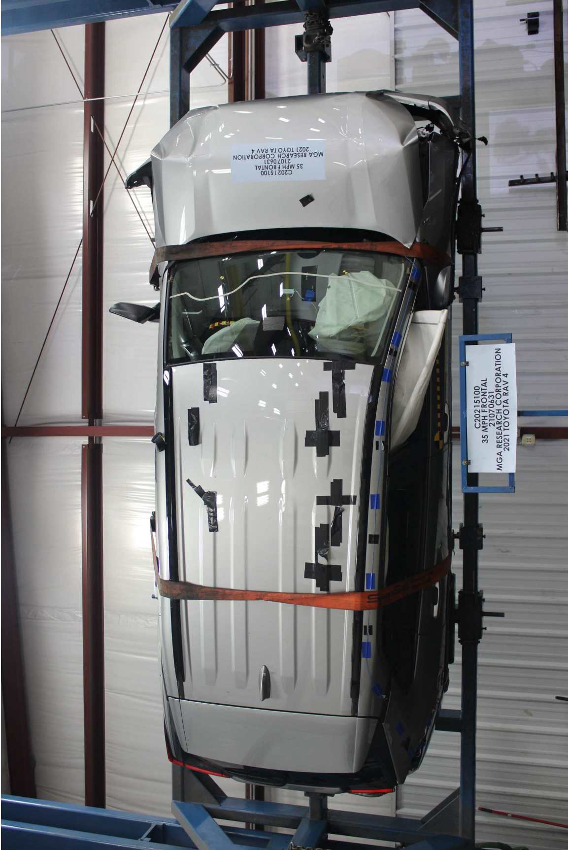
Photo No. 65. Rollover 270 Degrees
