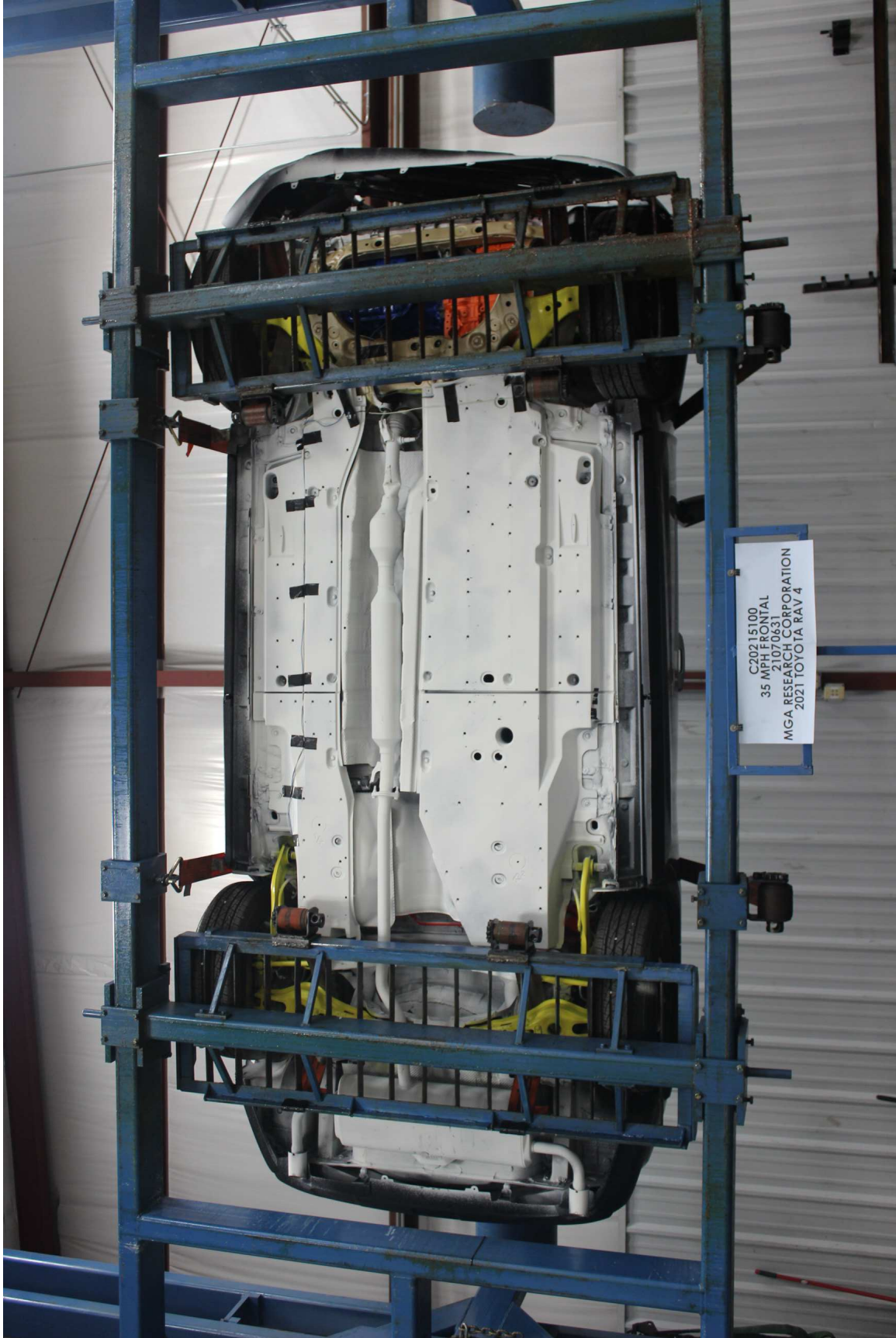
Photo No. 63. Rollover 90 Degrees
