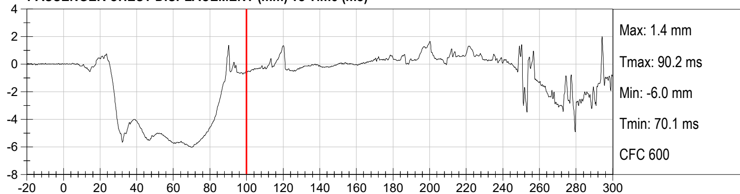
PASSENGER CHEST DISPLACEMENT (mm) vs Time (ms)
