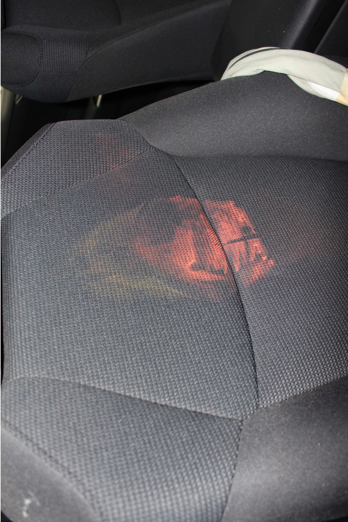
Photo No. 34 - Post-Test 6YO P1 Passenger Dummy Head Contact (seat back)
