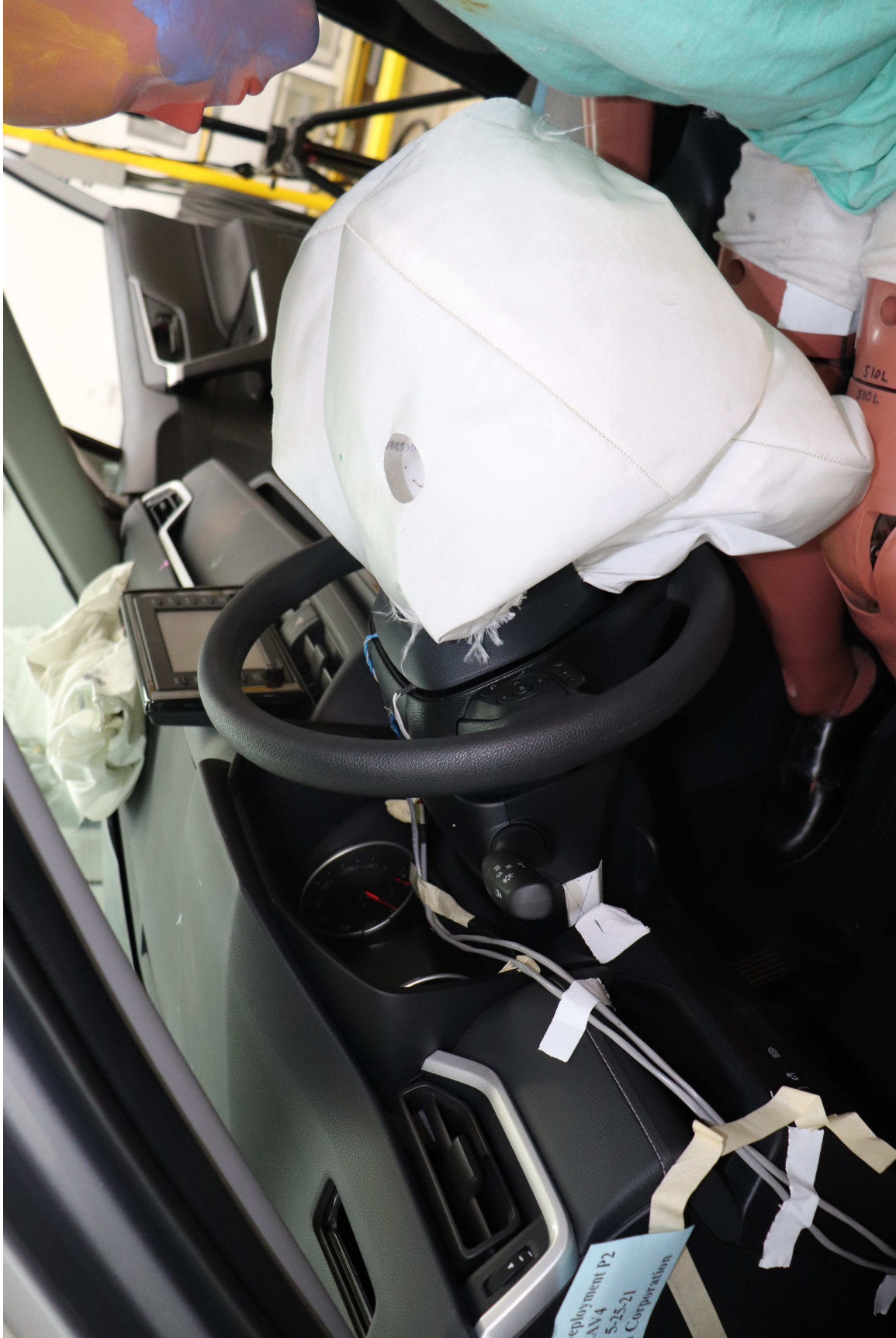
Photo No. 11 - Post-Test 5th Fem. P2 Driver Dummy Airbag Left Side View
