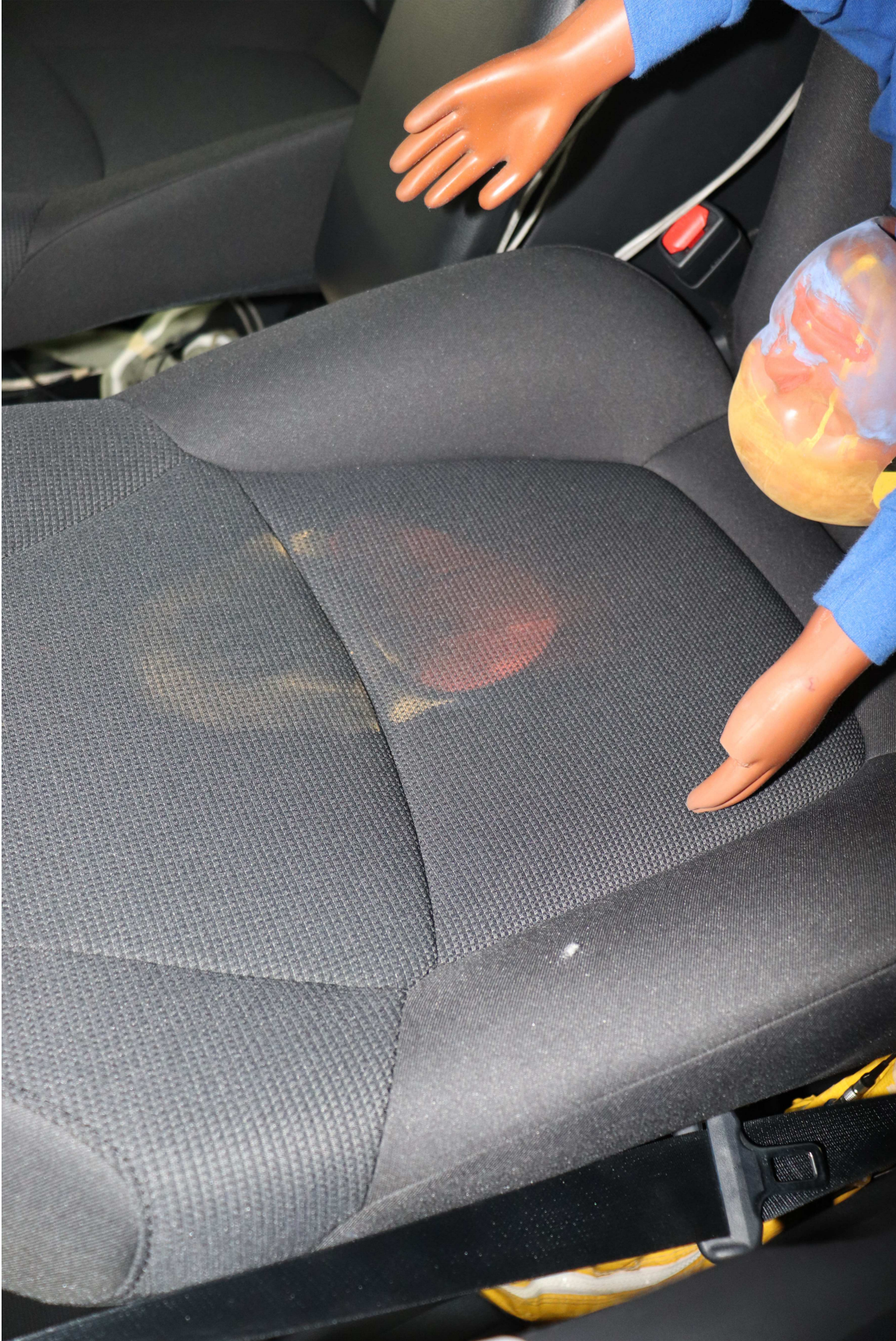
Photo No. 20 - Post-Test 3YO P1 Passenger Dummy Head Contact (seat back)
