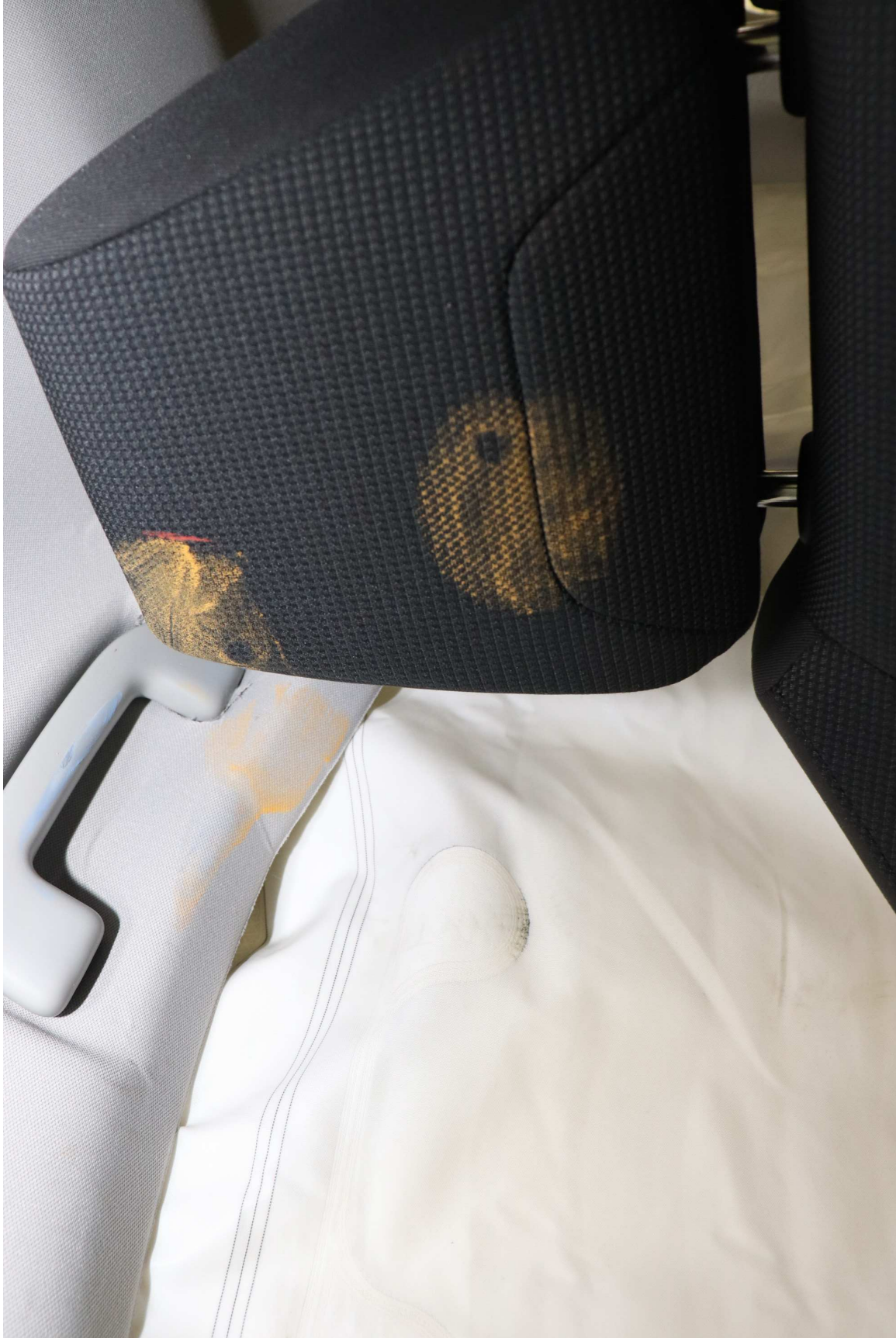
Photo No. 62. Post-Test Passenger Dummy Head Contact (headrest-headliner)
